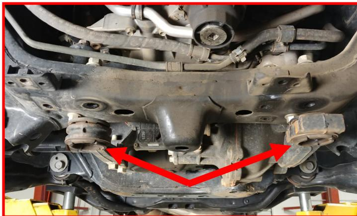
Install the ReadyLIFT differential drops in between the factory mounts and frame.
