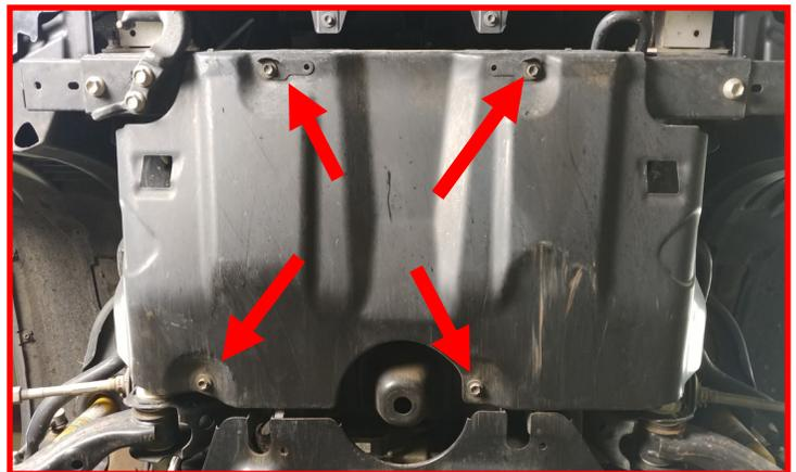
If equipped, remove the differential gravel guard.
