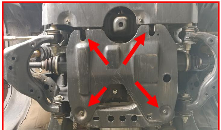
Locate the front gravel guard mounts on the frame. Look to see if there will be any clearance issues with the front differential mount when it is lowered. (Driver side shown.)
