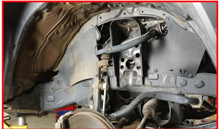
Install the ReadyLIFT strut extension to the strut using the **factory hardware**. Torque to **30 ft-lbs**.
