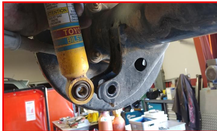
Working on one side at a time, loosen but do not remove the opposite side u-bolts of the side you are working on.
