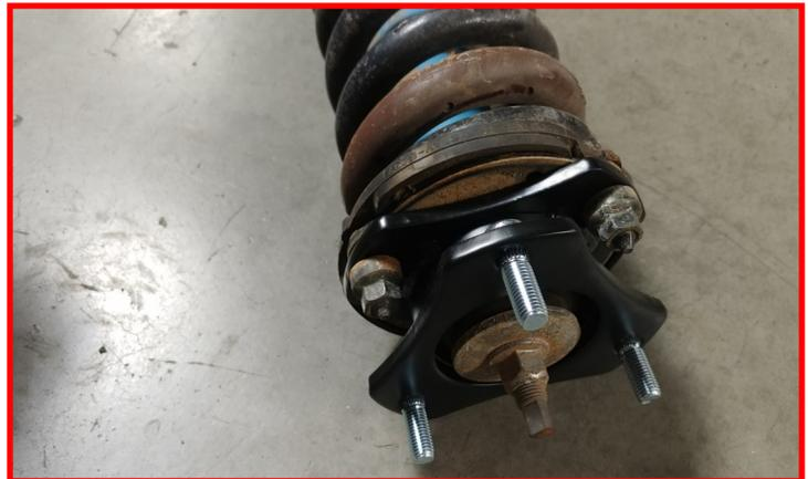
Install the completed strut assembly to the frame using the provided hardware. Do not tighten at this time.
