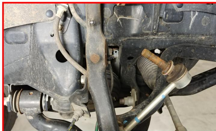
Remove the sway bar from the frame rail. Let hang out of the way.
