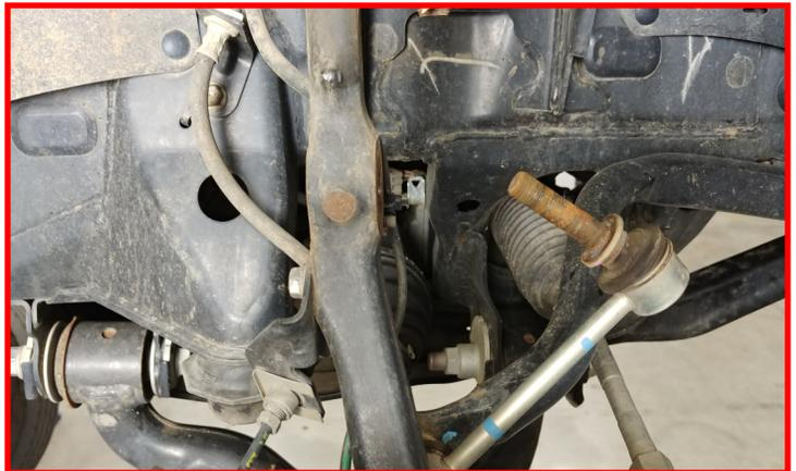
Remove the lower strut hardware.
