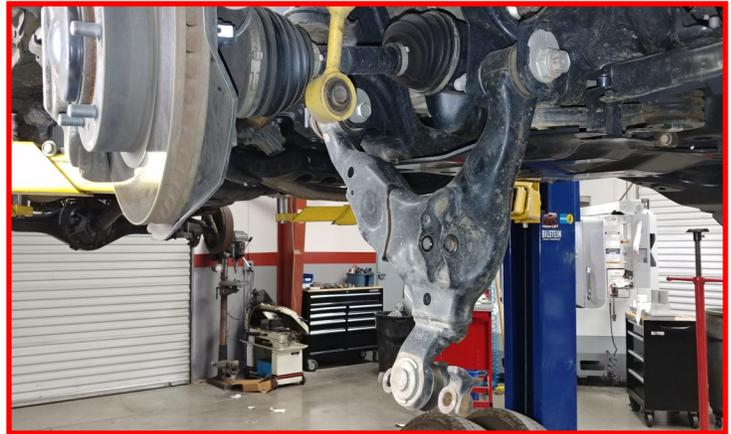
Remove the strut from the vehicle.
