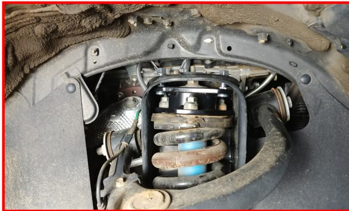
Raise the lower control arm up and install the lower strut hardware. Do not tighten at this time. Loosen but do not remove the upper control arm hardware to allow the bushings to relax and have the suspension droop out. Install the lower ball joint cradle to the knuckle using the **factory hardware**, and a drop of thread locker. Torque to **125 ft-lbs**.
