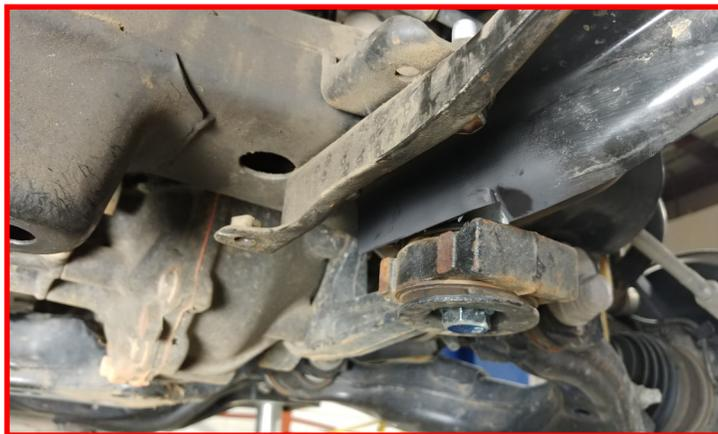
Install the previously removed passenger side gravel guard support using the **factory hardware**. Torque to **45 ft-lbs.** (Modified mount shown)
