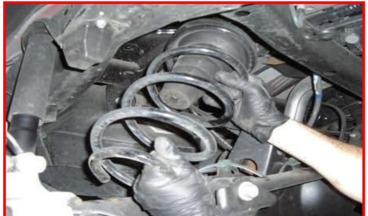
Install the ReadyLIFT spring spacer on top of the spring and rubber isolator. Install the assembly into the vehicle. Raise the axle up to hold the springs in place.
