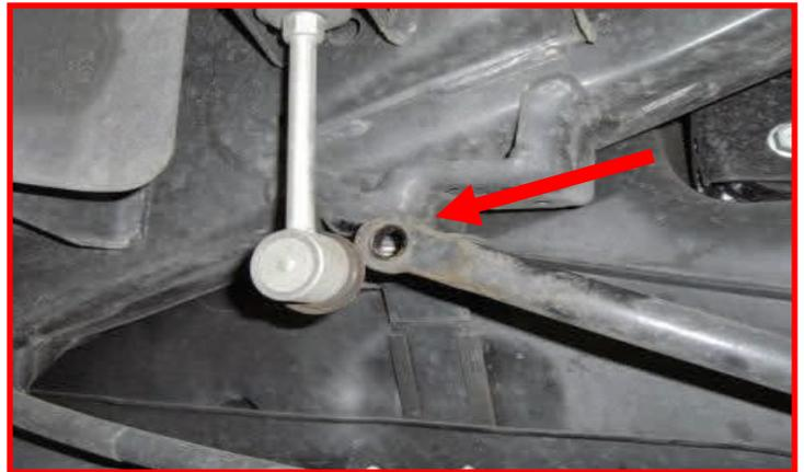
Lower the axle down enough to remove the springs and install the spacer. Be careful to not over extend any ABS or brake lines.
