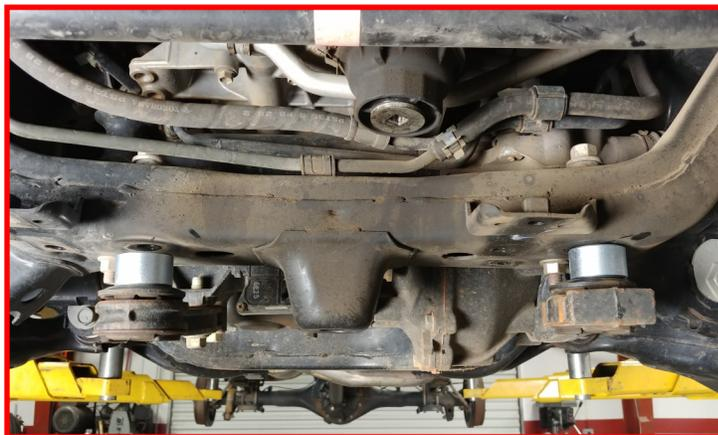
Install to the frame using the **provided hardware** and the **factory large bushing washers** in their original location. Torque to **95 ft-lbs.**
