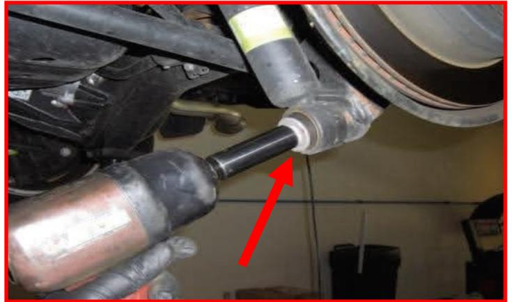
Disconnect the lower sway bar end link from the sway bar. Let the sway bar hang out of the way. Loosen but do not remove all control arms and track bar hardware.
