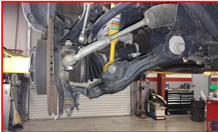
Install the sway bar end link to the knuckle using the **factory hardware**. Torque to **45 ft-lbs**.
